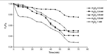
Fig. 2 Influence of the  $H_2O_2$  initial concentration on the dye conversion in the reactor. [AO7]—11.32 mg/l, HRP—1U/ml, pH 7, and temperature of 25 °C
