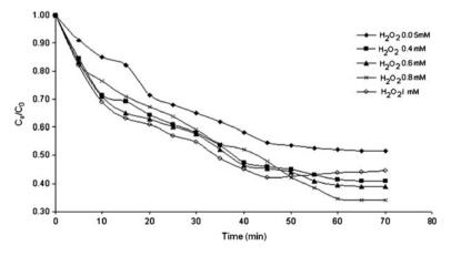
Fig. 3 Influence of the  $H_2O_2$  initial concentration on the dye conversion in the reactor. [AO7]—23.17 mg/l, HRP—1U/ml, pH 7, and temperature of 25 °C
