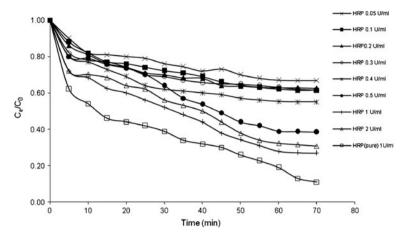
Fig. 1 Influence of the HRP initial concentration (0.05–2 U/ml) on the AO7 conversion in a batch reactor. AO7—11.32 mg/l, [H<sub>2</sub>O<sub>2</sub>]—1 mM, pH 7.4, and temperature of 25 °C
